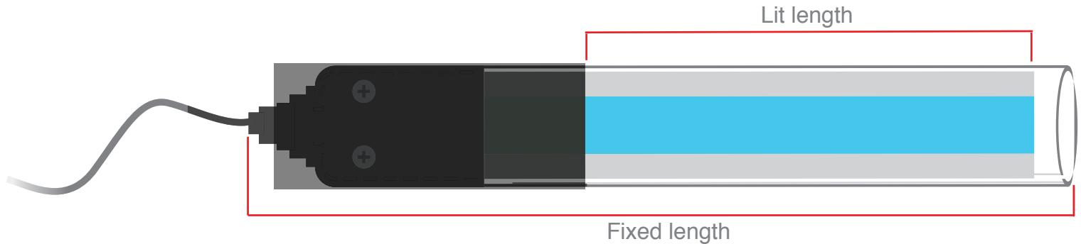
The 2" wide Light Tape® Snap-N-Light™ system employs two connection points for optimal performance. Please allow an additional 5.5" when determining the dimensions of your Light Tape's Snap-N-Light™ system. This 5.5" accounts for 4.5 inches for the Light Tape® Connector and strain relief, 1/2" for wire flex, and 1/2" for the area between the end of the lit area and the end of the extrusion.
