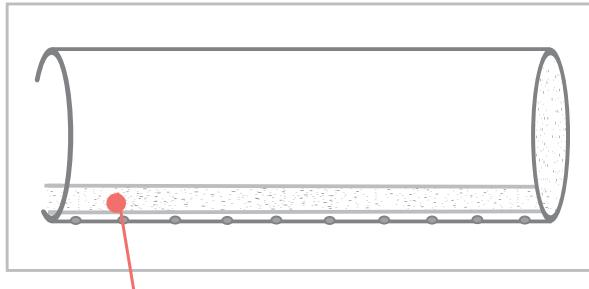
**2** Make sure drain slot is located at the bottom to allow for drainage. **DO NOT** fill open ends of the extrusion with silicone. If mounting with an adhesive do not block bottom gap.
