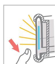
Press firmly downward to snap in place, making sure that slit in back is not covered to allow for drainage.
